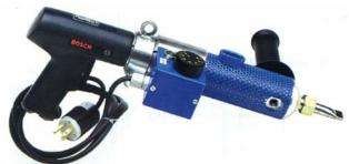
A lighter-weight, hand-held extruder gun for filling skived repair areas with hot flowing repair rubber. Ideal for truck and O.T.R. tyre repairs. Cuts material waste and eliminates trapped air. Adjustable thermostat holds set temperature. Air operated, requires 90-100 psi.
